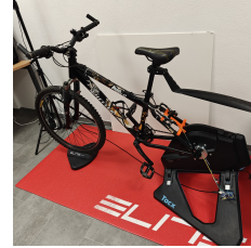
Fig. 3. Hardware setup of the bicycle simulator consisting of an ordinary bicycle where the rear wheel is replaced by a bike trainer. The cyclist wears VR glasses (not shown) to experience the virtual world.
