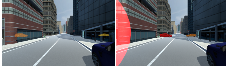
(b) The Bicycle Warning System (BWS) prototype: Vehicles highlighted with color-coded overlays (yellow = attention, red = critical), independent of gaze direction.
