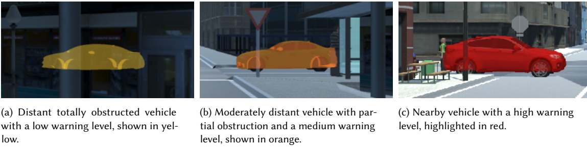
Fig. 2. Color-coded warning overlays used in both Bicycle Warning System to indicate the perceived threat level of approaching vehicles based on distance and visibility.
