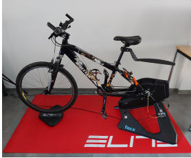
(a) Bicycle simulator setup. Cycling speed was tracked with a Tacx Neo 2, steering via an Elite Sterzo Smart, and visuals with a Varjo Aero VR headset.
